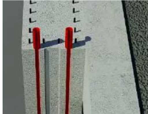
The guide track system ensures full-width contact between jointed elements
